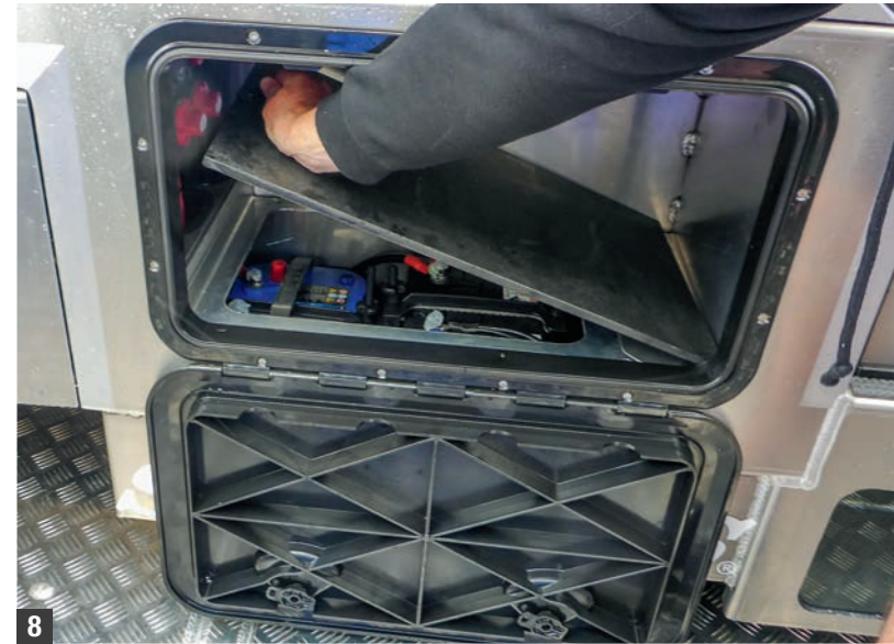
5) Footrests are incorporated into storage racks against the cabin bulkhead with the larger one on the passenger side. 6) Surtees boats provide a soft ride in rough conditions. 7) Catch storage is sorted with an aftermarket ice bin. 8) A central locker houses the dual battery system under a false floor.
