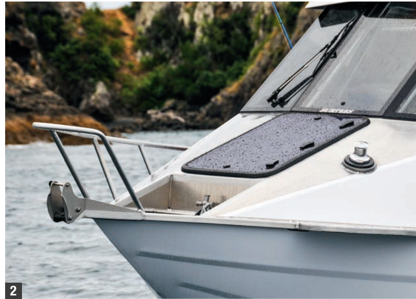
1) The forward cabin has a lockable sliding door for secure gear storage. 2) The ground tackle comes up over the fairlead, then runs up to an anchor capstan on the outside of the cabin. 3) The transom step-through with drop door aligns with the fold-down boarding ladder. 4) A locker on the starboard side incorporates the fuel filter and forms a fold-down single bench
