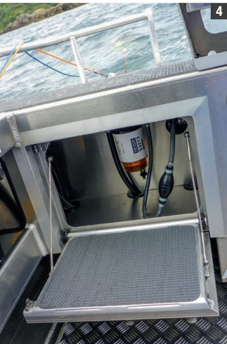
1) The forward cabin has a lockable sliding door for secure gear storage. 2) The ground tackle comes up over the fairlead, then runs up to an anchor capstan on the outside of the cabin. 3) The transom step-through with drop door aligns with the fold-down boarding ladder. 4) A locker on the starboard side incorporates the fuel filter and forms a fold-down single bench
