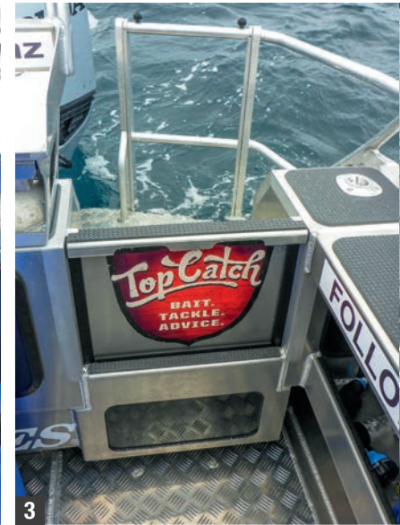
1) The forward cabin has a lockable sliding door for secure gear storage. 2) The ground tackle comes up over the fairlead, then runs up to an anchor capstan on the outside of the cabin. 3) The transom step-through with drop door aligns with the fold-down boarding ladder. 4) A locker on the starboard side incorporates the fuel filter and forms a fold-down single bench
