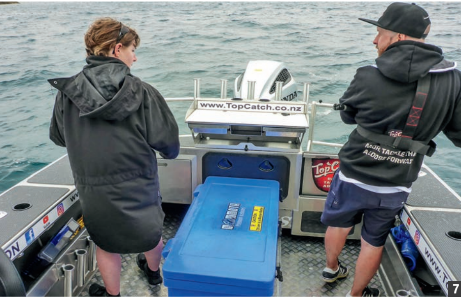
5) Footrests are incorporated into storage racks against the cabin bulkhead with the larger one on the passenger side. 6) Surtees boats provide a soft ride in rough conditions. 7) Catch storage is sorted with an aftermarket ice bin. 8) A central locker houses the dual battery system under a false floor.
