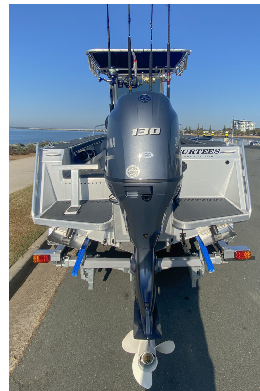
Yamaha's F130 was the power plant for this boat, although the rig is rated to 150hp.
