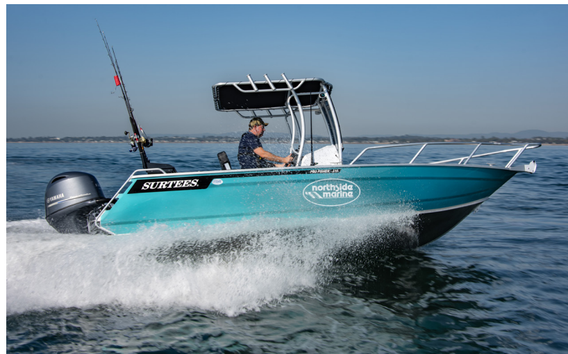
Top: Best economy was at 3,900rpm, where the Yamaha delivered 2.4km/L at 36km/h. Above: Open up the throttle and the economy drops to 1.4km/L, but you race along at 64km/h.
