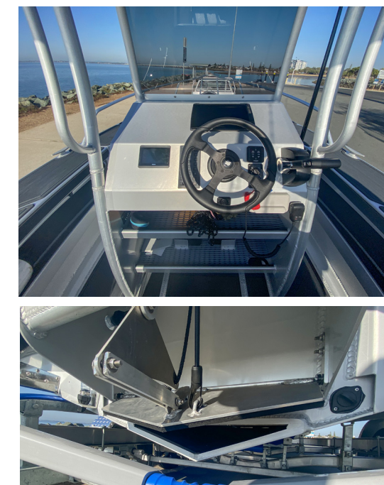
Top: A wide console gives more protection from the elements and check out all of that space to mount your MFDs. Above: Here's the entry to the water ballast system. Close the flap and you've trapped hundreds of litres of water in the keel and the ride will benefit from the extra mass.
